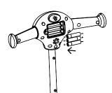
2. Open battery door compartment and insert three new AAA (1.5V) Alkaline batteries. Be sure to insert with correct polarity.
