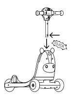
2A. Insert handle with the Horn/Light Button facing FRONT. Press in lower button while pushing handle down until it clicks.
