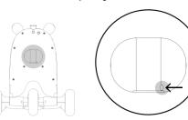
3. Re-insert front wheels with the "locator" in the BACK. Check the window to make sure the metal button is visible on the LEFT side.
