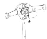
1. Loosen the battery door screw using a Philips head screwdriver.
