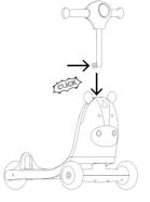
**4A.** Insert handle with the Horn/Light Button facing the BACK. Press in lower button while pushing handle down until it clicks.
