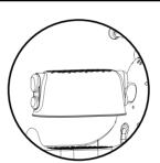
1. Remove seat while pressing release buttons.
