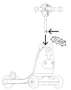
2A. Insert handle with the Horn/Light Button facing FRONT. Press in lower button while pushing handle down until it clicks.
